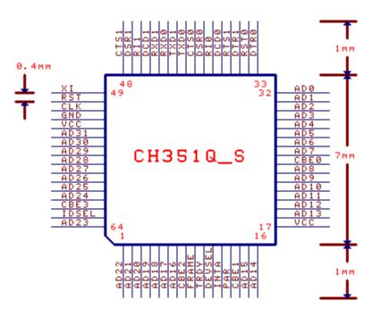
Refer to the Datasheet (II) CH351DS2.PDF for the application instructions and pins diagram of parallel/ printer port.
