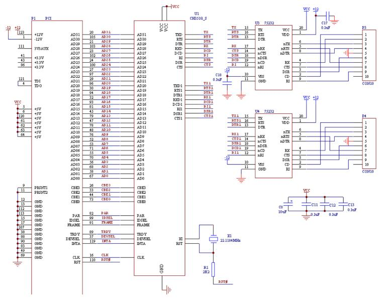
This is a PCI dual-channel serial port circuit based on the CH351. U3 and U4 are RS232 conversion chip 75232, P3 and P4 are 10-pin double-row or DB9 pins. Crystal X1 is used for the clock oscillation circuit. Capacitor C0 and C11 $\sim$ C13 are used for power decoupling, C11 $\sim$ C13 are monolithic or high-frequency ceramic capacitors with a capacity of 0.1uF. They are connected in parallel nearby to the power pins of
